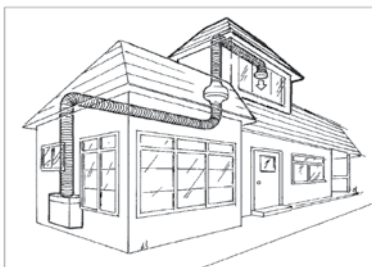
(AIF Fan) transferring conditioned air to a new room addition
